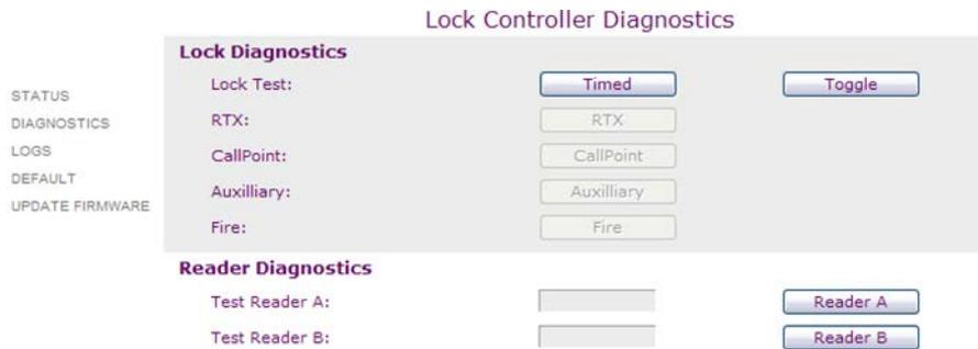
The diagnostics page allows you to simulate any condition at the door remotely. The following diagnostic functions are available:
