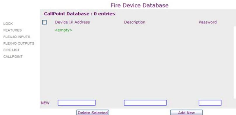
The database contains the IP addresses of the devices to be notified in the event of fire alarm activation. The database must be populated manually.
